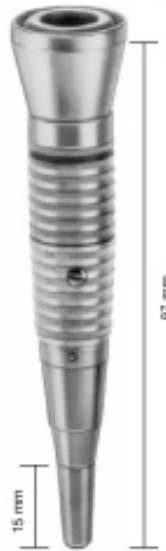
M8-201 INTRA Main Piece, Straight No key needed for tightening Tip 15 mm long Transmission: 1:1 Color marked: Blue Burs shank: Ø 2.35 mm Burs length: 70 mm
