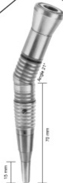
M8-210 INTRA Main Piece, Angular No key needed for tightening Tip 15 mm long Transmission: 1:2 Color marked: Red Burs shank: Ø 2.35 mm Burs length: 70 mm
